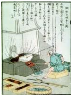
Around 1600 Perfected nanban-buki, a copper refining technique for separating silver from copper ore containing silver
