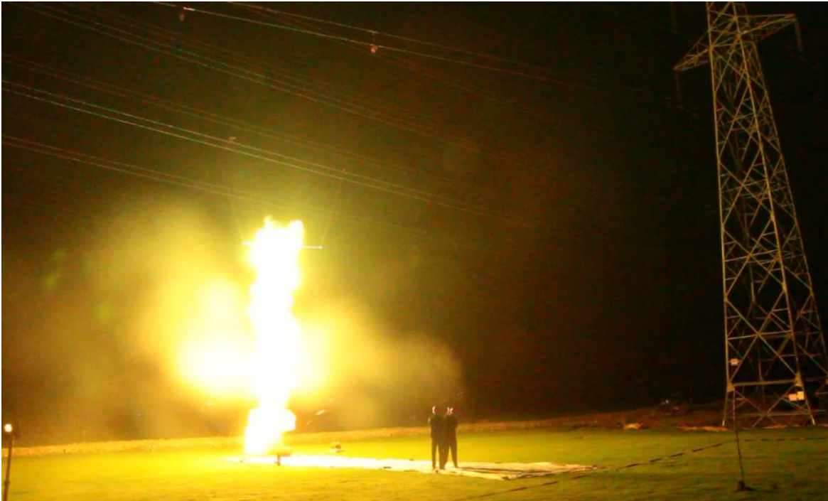
Artificial AC fault test on site
