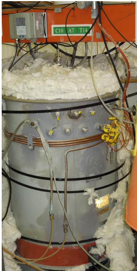
FIGURE 4: 100 KVA DISTRIBUTION TRANSFORMER USE FOR THE MARKERS TEMPERATURE EQUILIBRIUM TEST
